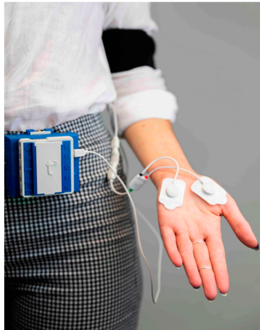
Figure 6. Electrodermal activity (EDA) sensors and the BITalino box.
